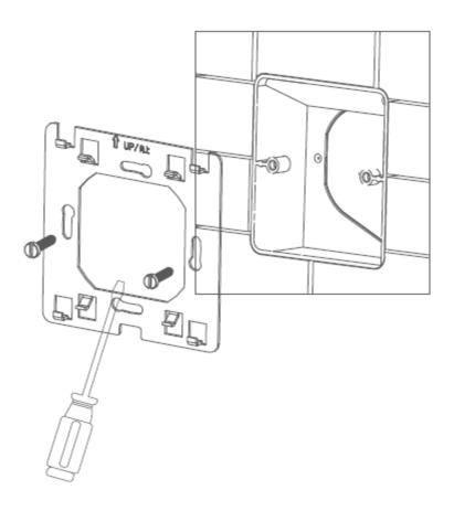
4. After connecting wires (see connecting diagram), mount the thermostat on the backing plate and remount the cover and frame.
