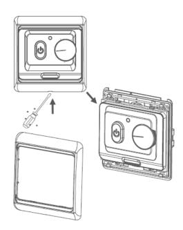
2. Take the backing plate apart according to the following diagram.
