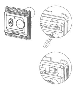
3. Mount the backing plate in the wall socket by screwdriver. The thermostat is installed in standard wall boxes with 60mm between the screws.
