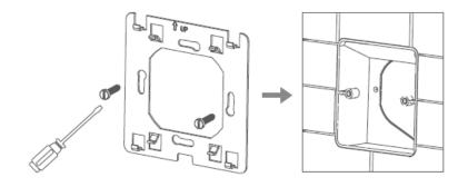
4. After connecting the wires, mount the controller on the back and remount the cover and frame.
