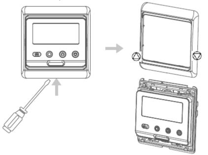
2. Take the back plate apart according to the below diagram.
