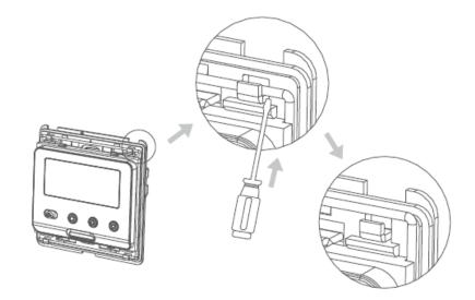
3. Mount the back plate in the wall socket by screwdriver. The thermostat is installed in standard wall boxes with 60mm between the screws.
