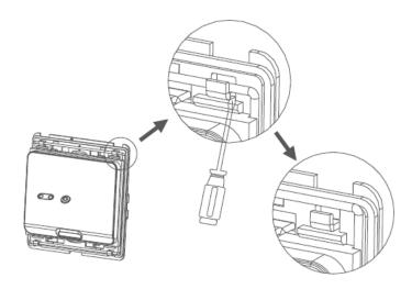
3. Mount the backing plate in the wall socket by screwdriver. The thermostat is installed in standard wall boxes with 60mm between the screws.
