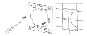
4. After connecting wires (see connecting diagram), mount the thermostat on the backing plate and remount the cover and frame.
