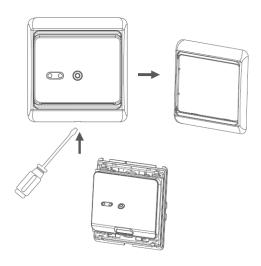
2. Take the backing plate apart according to the following diagram.
