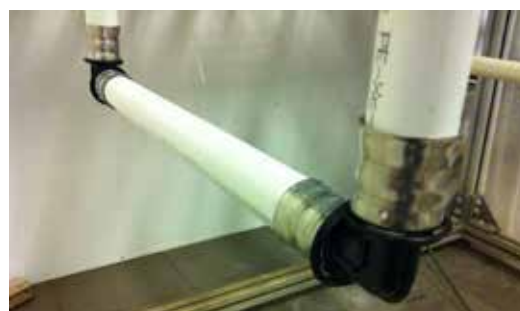
TERMAL CYCLING TEST AC-FIX PRESS DUO (PPSU) WITH MULTILAYER PIPES
