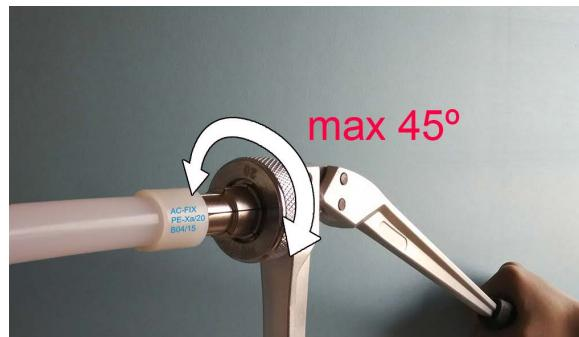
4. Gradually press the handles together fully. On 20mm and larger pipe sizes, keep the handles together for around 3 seconds.
