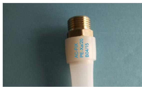
5. Open the handles, remove the expander tool and directly push the pipe onto the fitting nipple. The plastic ring on the pipe end must reach entirely the shoulder.
