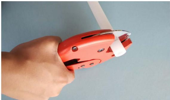
1. Cut the pipe as clean and perpendicular as possible to its axis.
